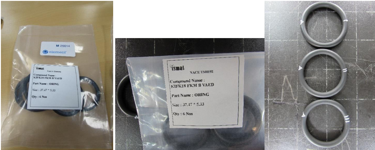
Figure A.1: As received material/before start of RGD: KIFK18 FKM B VAED
